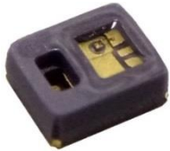
Single Aperture Combo Light Sensor (ALS/RGB+PS) 2.5x2.0mm
